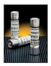
GFN midget indicating fuses are available in ratings from 1/10A through 30A. These time-delay fuses have built-in blown fuse indicators which pop out at the end of the fuse to visually indicate when the fuse has operated to open the circuit. Indicators may be used to trip a switch for remote as well as visual annunciation. (Not for Branch Circuit Protection).
